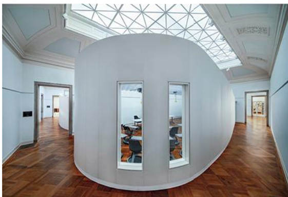
Landmarked galleries of the Corcoran School of the Arts & Design were outfitted with learning spaces designed to be reversible, per historic preservation guidelines.
